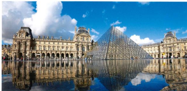
Photocatalysis acts as an antifouling and antifogging effect simply by the irradiation of light. It has also been used in the glass covering the pyramid-shaped entrance of the Louvre Museum. The glass maintains its transparent beauty by decomposing dirt.
